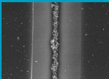
An electron microscope image shows a sub micron wire assembled in a silicon V-groove.
