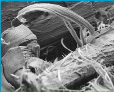
A scanning electron micrograph image of a fracture surface of a harakeke-epoxy composite. The finest filaments are individual macrofibrils torn from the fibres, and suggesting resin penetration into cell walls has occurred.
